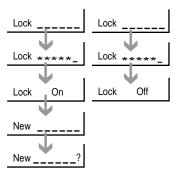
2 Input the correct password. (6-digit, the preset password is 123456). After inputting, the screen displays "Lock: On".
